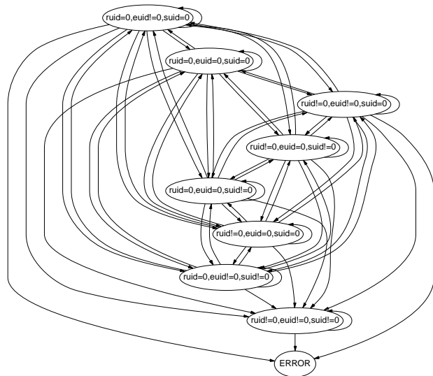
Figure 9: A refined view of the Linux 2.4.17 process privilege model, capturing the ruid , euid , and suid .
